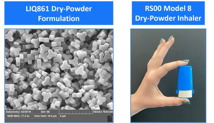
LIQ861 particles are 1.2 µm in size with trefoil shape
